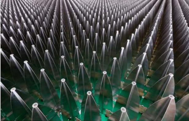
Fig. 2 Photograph of the EMBRACE antenna array
