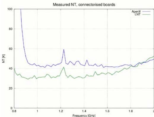
Fig. 3 Low Noise Tile (LNT) receiver noise measurements
