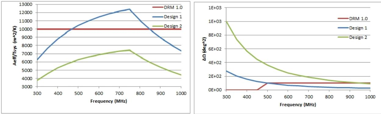
Figure 2. Effective Area divided by  $T_{\text{sys}}$  (left) and field-of-view (right) function of frequency for two designs
