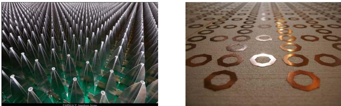
**Figure 3. The candidate antenna technologies for MFAA, Vivaldi (left) and ORA (right)**
