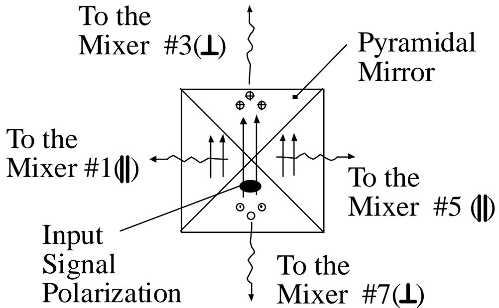
**Figure 5:** Schematic of the pyramidal mirror as viewed from above. Each mixer receives the polarisation orthogonal to that of its neighbour. Mixers #1 and #7 should have their polarisation axis orientated at  $90^\circ$  to that of mixers #3 and #5.
