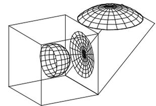
**Figure 4** Each mixer unit incorporates a 90/10 beam splitter with an absorber below to take the unused LO power, and a lens above to couple the LO into the mixer
