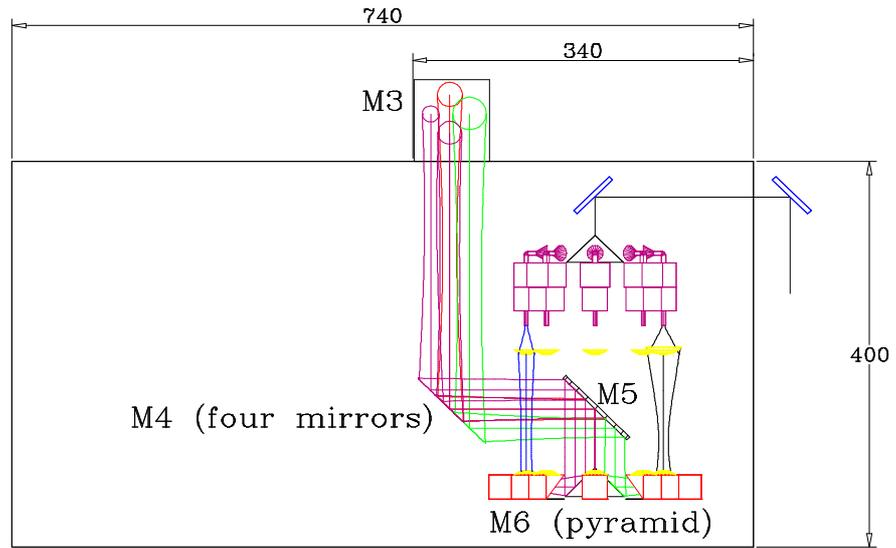
**Figure 2:** The side view of the HET design shows some dimensions indicating that the entire system fits into less than 50% of the volume presently reserved for this instrument.
