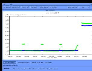
**Fig. 8 (left)** In the data reduction tool, one can plot the mean values of consecutive spectra. Here, Odin was using the "Sky Switching" observing mode. Alternate blue and green points show the "on" and "off" positions. The three clusters of high green points are the integrations in the internal calibration load. At the end of the sequence, Odin begins to observe the Earth's atmosphere.
