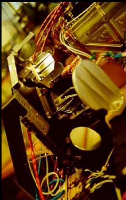
**Fig. 2 (left)** The main optics plate of the *Odin* radiometer just before integration into the satellite.
