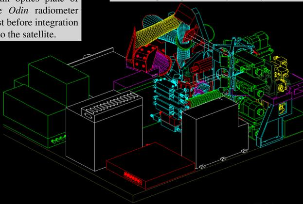
**Fig. 3 (below)** A CAD drawing of the *Odin* radiometer platform showing the 3-dimensional quasi-optical ray tracing that was used to help design and analyse the system.
