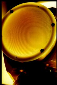
**Fig. 4 (left)** A teflon lens for the 119GHz receiver has linear matching grooves to eliminate reflections
